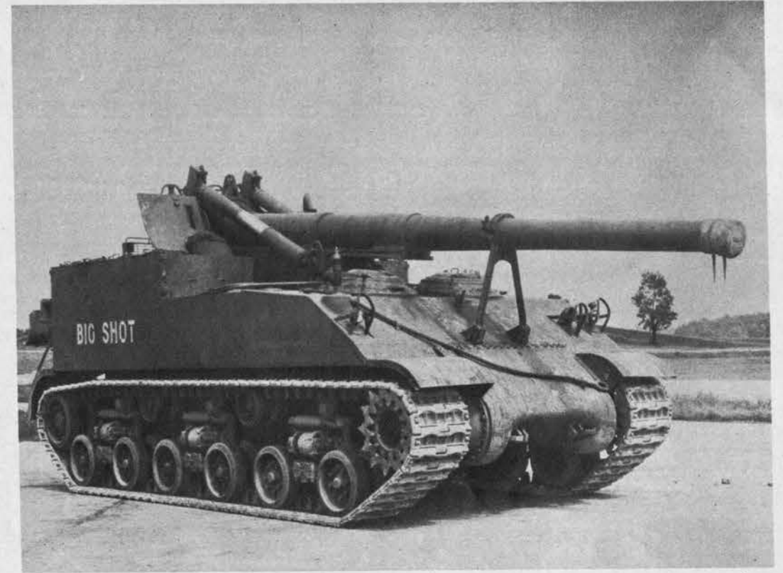
New M-4 suspension , the horizontal volute, is used on latest 155-mm. gun motor carriage, T-83. It has a broad track, prominent return rollers and horizontal springs between bogie wheels.
